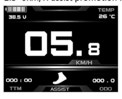
Hold and flashes, the vehicle drives at the speed not more than 6Km /h. Release button, the function is invalid.
