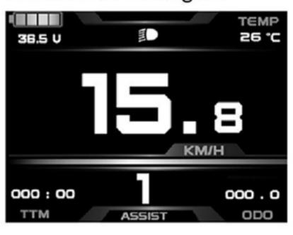
Hold long to turn on headlights (the controller should have headlight drive output function); hold long again to turn off the headlights.
