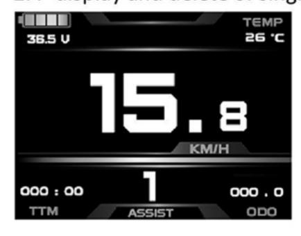
After power on for 5 seconds, hold and at the same time, single trip riding time (TIM) and single trip distance (DST) flash, hold button shortly, the content of both is cleared. If failed holding the button within 5 seconds, it will automatically return the display interface after 5 seconds, original content is preserved.
