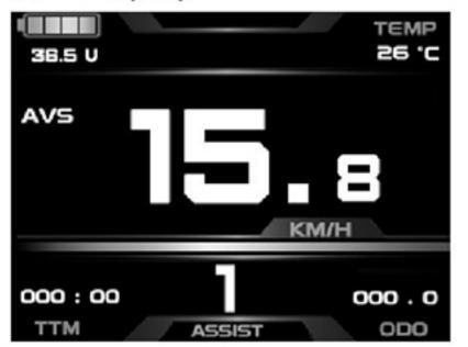
Press button in display 1 to enter display 2. In the riding mode within 5 seconds, display 2 automatically returns to display 1.
