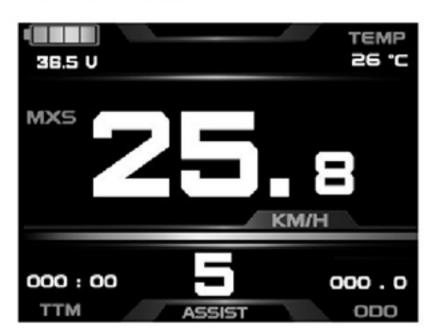
Press button in display 2 to enter display 3.In the riding condition, 5 seconds later, a single maximum speed (MXS) display automatically returns to the real riding speed (Km/H).
