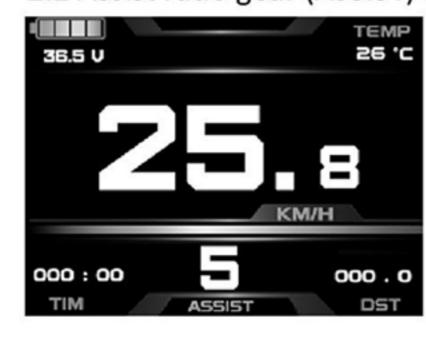
Press or to switch 0-5 file gear. Gear 1 is for the minimum power, gear 5 is for the highest power. Each startup will automatically restore the gear shutdown last time (the user can set randomly). Gear 0 is without booster function.
