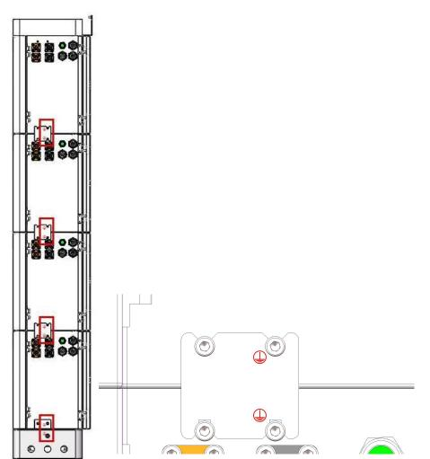
**Step 9**Connect to the power and communication cable.
