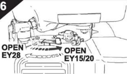
After starting the engine, gradually open choke by turning the choke lever and finally keep it open fully.
